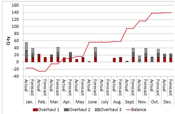
Fig. 2. Execution of forecast (moving average method) for spare compressor blades first stage.
