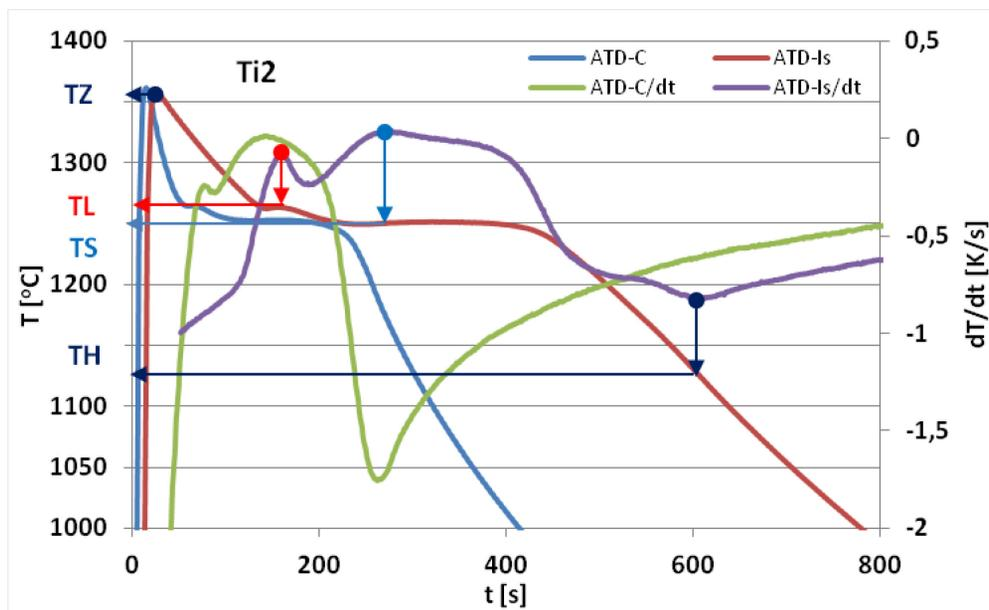
Fig. 5. TDA curves of Ti2 melt
