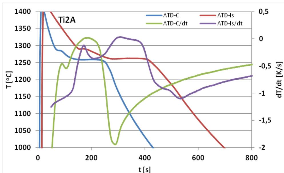
Fig. 7. TDA curves of Ti2A melt
