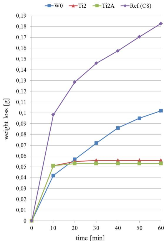
Fig. 9. Weight loss of samples in wear measurement cycles
