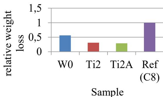
Fig. 10. Relative weight loss of examined samples in comparison to the wear test reference sample (C8)
