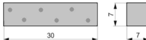
Fig. 2. Scheme of wear test sample with hardness measurement points
