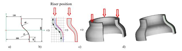
Fig. 3. Design of the casting using the module "CastDesigner" based on the "track curve" a) Sketch of the surface contour of the casting which was developed with the module "Sketch FreeCAD", b) Analysis of the feeding ability
