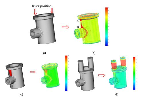
Fig. 7. Construction of the additional feeding path in the connection of the thermal knots a) Determining of the feeding direction, b) Inquiry of two thermal knots with the help of the 3D-analysis, c) Inquiry of the geometrical change to the union of both thermal knots taking into account of α – value, d) Inquiry of the riser and final check
