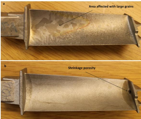
Fig. 1. Common defects in casting of turbine blades
