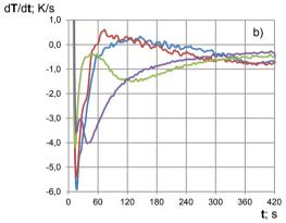
Fig. 5. Cooling curves recorded for the step block cast from melt H1 by four thermocuples placed at different locations in the mold corresponding to four steps with the wall thickness: g1=6 mm, g2=11 mm, g3=23 mm, g4=40 mm;
