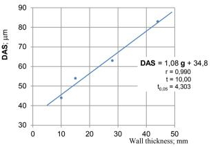
Fig. 12. Wall thickness effect on DAS in a casting made from the H282 alloy
