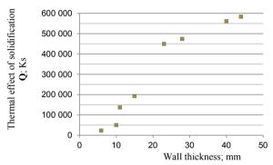
Fig. 10. Thermal effect of solidification as a function of wall thickness in casting made from the H282 alloy (data from melts H1 and H3 were used)
