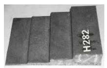
Fig. 4. Step g x 35 x 150 mm H282 alloy casting used in the conducted tests; g denotes the thickness of each "step"
