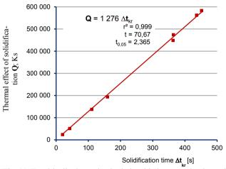
Fig. 11. Empirically determined relationship between the thermal effect of solidification  ${\bf Q}$  and the solidification time  $\Delta t_{kr}$  for H282 alloy (data from melts H1 and H3 were used )
