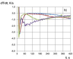
Fig. 6. Cooling curves recorded for the step block cast from melt H3 by four thermocuples placed at different locations in the mold corresponding to four steps with the wall thickness: g1=10 mm, g2=15 mm, g3=28 mm, g4=44 mm;
