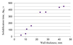
Fig. 9. Solidification time as a function of wall thickness in casting made from the H282 alloy (data from melts H1 and H3 were used)
