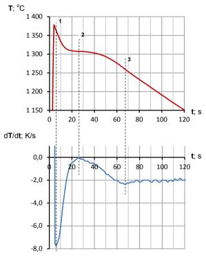
Fig. 1. A method to determine the characteristic parameters of the H282 alloy solidification process: a) base curve T = (t), b) differential curve dT/dt = f(t), where T - temperature,
