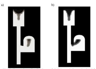
Fig. 3. Exemplary distributions of shrinkage defects obtained for the same casting geometries (traditional feeders): a – steel, b – grey cast iron
