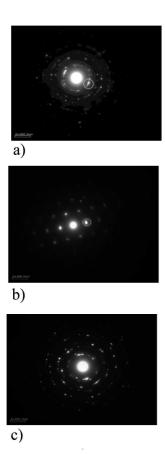
Fig. 13. Structure of the AlMn1Cu alloy (performed methods of SAED), a) initial state, b)  $5^{th}$  pass, channel without deflection, c)  $5^{th}$  pass, with  $10^{\circ}$  helix
