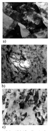
Fig. 12. Structure of the AlMn1Cu alloy (performed methods of TEM), a) initial state, b)  $5^{th}$  pass, channel without deflection, c)  $5^{th}$  pass, with  $10^{\circ}$  helix
