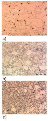
Fig. 11. Results of metallographic analysis of the magnesium alloy AZ31, a) initial state, b) 3rd pass, c) 5th pass
