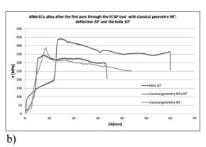
Fig. 8. Stress-strain curves a) after the first and b) after the fifth pass through ECAP
