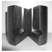
Fig. 5. ECAP tool with helix matrix
