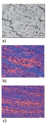
Fig. 10. Results of metallographic analysis of the AlMn1Cu alloy a) initial state, b)  $3^{rd}$  pass, c)  $5^{th}$  pass
