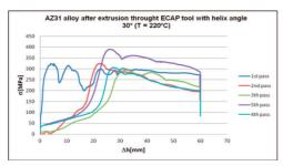
Fig. 9. Stress-strain curves ECAP with helix matrix
