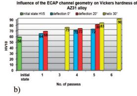
Fig. 14. Results of hardness, a) AlMn1Cu alloy, b) AZ 31 alloy
