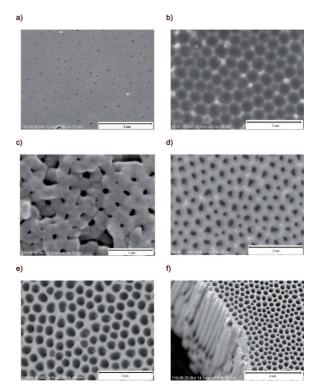
Fig. 5. SEM images of the membrane after each of the process stage: a – after the first stage of anodizing, b – after the removal of  $Al_2O_3$ , c – after the second stage of anodizing, d – after the widening of pores e – after the removal of the barrier film f – the membrane prepared for cathodic deposition of Co-Fe nanowires
