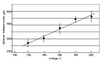
Fig. 3. The relationship between the distance between pores and the electrolysis voltage; anodizing conditions: 0.17 M  $H_3PO_4$  solution, time 24 h, temperature 1°C
