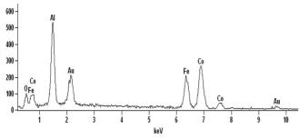
Fig. 8. The EDXS analysis of the chemical composition of the membrane containing Co-Fe nanowires
