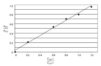
Fig. 7. The relationship between the ratio of the number of moles  $(n_{Fe})/(n_{Co})$  of both metals in the cathodic deposit (Co-Fe alloy) and the ratio of the concentrations of ions  $(C_{Fe2+} / C_{Co2+})$  in the electrolyte
