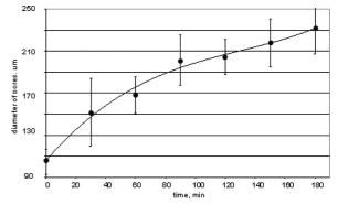
Fig. 4. The influence of the chemical treatment time on the diameters of pores in  $Al_2O_3$  membranes; anodizing conditions: 0.17 M  $H_3PO_4$  solution, temperature 1°C, the voltage 180 V
