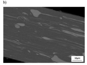
Fig. 6. Microstructure of CuNb wire after rolling and drawing  $\varphi$  90  $\mu$ m, a) cross section, b) longitudinal section
