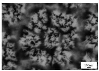
Fig. 9. Microstructure of CuNb composite wire after 7th bundling, diameter  $125 \mu$ m, magnification: a) 1 300x, b) 30 000x, c) 100 000x
