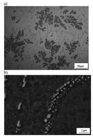
Fig. 4. Microstructure of CuNb ingot, a)optical microscopy, b) SEM
