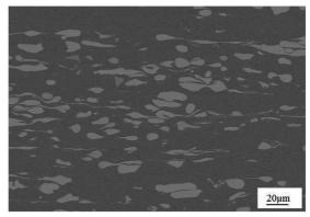
Fig. 5. Microstructure of CuNb wire after rolling and drawing  $\varphi$ 2,8 mm, a) cross section, b) longitudinal section
