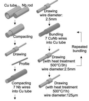
Fig. 3. Processing of CuNb microcomposites (bundling method)
