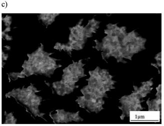
Fig. 8. Microstructure of CuNb composite wire after 7th bundling, magnification: a) 35x, b) 3 000x, c) 22 000x
