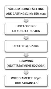
Fig. 2. Processing of CuNb microcomposites (classical method)
