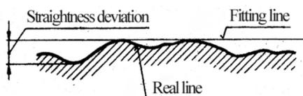
Fig. 2. Straightness deviation
