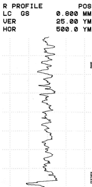
Fig. 5. Casting surface roughness profilogram from Fig. 1
