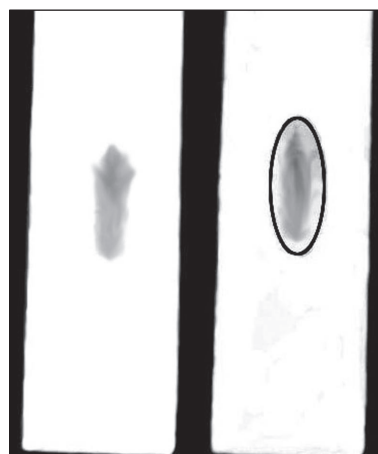
Fig. 6. TLC plate of the phytotoxic fraction, circle shows the blue spot ( R_f : 0.5–0.6)
