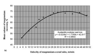
Fig. 2. Magnesium recovery mean values as a relation to the range of optimized temperature of molten alloy treatment a) and their trend as a relation to the velocity of a magnesium-cored wire b)
