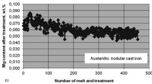
Fig. 1. Optimization of the length of nodulariser wire a), treatment temperature b) and residual magnesium content c) carried out during experiments of austenitic nodular cast iron (EN-GJSA-XNiSiCr35-5-2 Grade)
