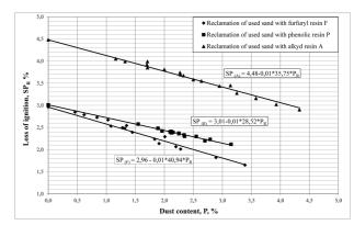
Fig. 1. Accumulated dependence of the reclaimed matrix ignition losses, after the pneumatic classification, on the dusts content generated during the reclaim treatment of three kinds of spent moulding sands in the rotor tester AT-2
