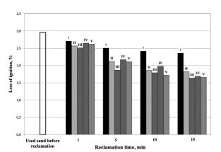
Fig. 4. Ignition loss values of the matrices reclaimed in the recycling process performed according to I-V methods
