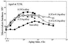
Fig. 1. Age-hardening curves of alloys aged at 523 K
