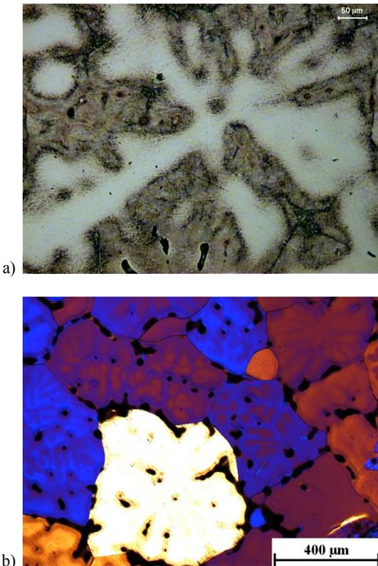
Fig. 2. The AlZn20 alloy microstructure image; (a) initial unmodified, (b) modified with (Al,Zn)-Ti3 MA, introducing 0,04 wt% Ti to the solution [6]
