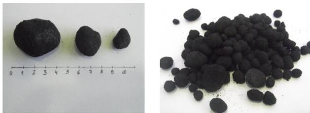
Fig. 3. Granulate fractions, granulator rotational speed – 10 rpm, angle of inclination –  $40^\circ$ , scale in cm
