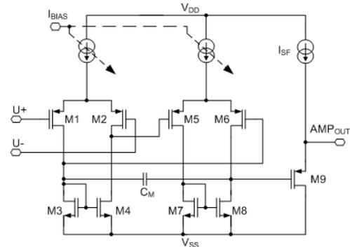
Fig. 3. Simplified scheme of the AMP1.
