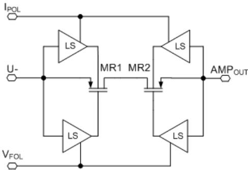
Fig. 4. Simplified scheme of the AMP1 resistive feedback.
