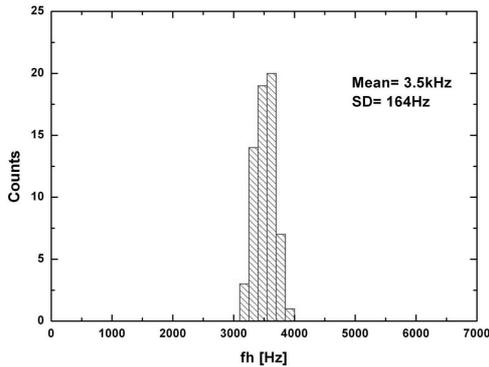
Fig. 8. Distribution of the high cut-off frequency for  $V_{FOL} = -0.2V$ .
