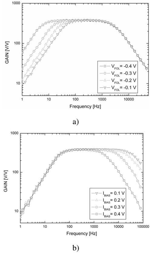
Fig. 5. Frequency response of single channel: a) low cut-off frequency tuning, b) high cut-off frequency tuning.
