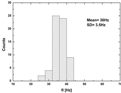
Fig. 7. Distribution of the low cut-off frequency for  $V_{FOL} = -0.2V$ .
