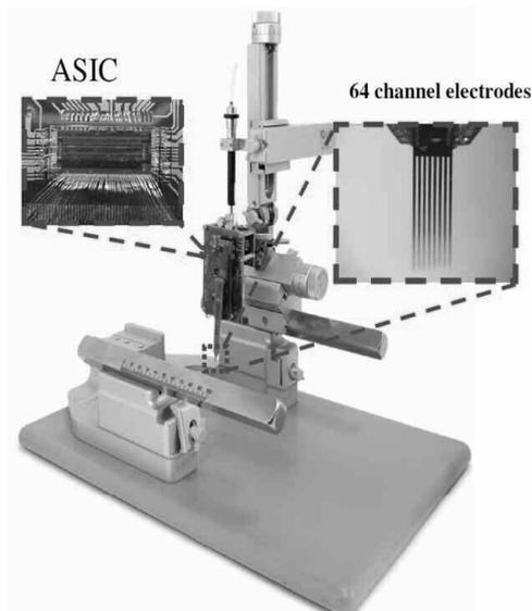
Fig. 14. 64 channel system for in vivo experiments.
