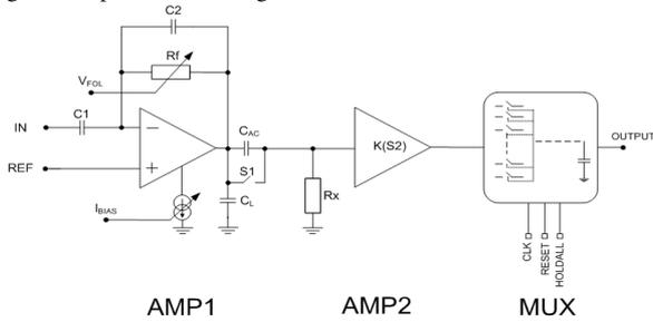
Fig. 2. Simplified block diagram of single readout channel.
