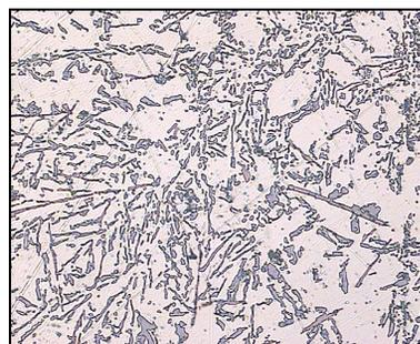
Fig. 3. Structures of AlSi11 alloy without modification (conventional moulding material with oil binder)
