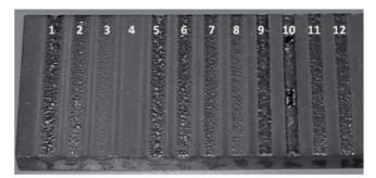
Fig. 3. Macroscopic effects of remelting
