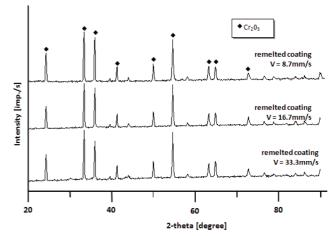
Fig. 8. Results of the X-ray phase analysis of oxide coatings as a function of applied remelting parameters
