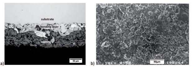
Fig. 4. Structure and morphology of plasma sprayed coatings: a) cross-section - light microscope and b) surface, SEM
