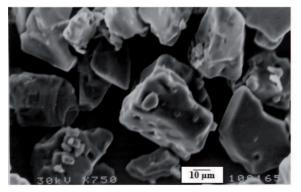
Fig. 1. Structure of the  $Cr_2O_3$  powder used in the plasma spraying process, SEM
