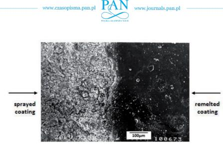
Fig. 6. Border between the sprayed and remelted surface (SEM)
