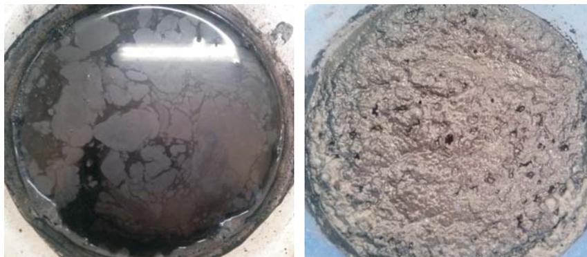
Fig. 4. Foam images using air bubbles (on the left) and oily bubbles (on the right)
