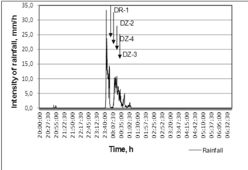
Fig. 7. Rainfall hyetograph with marked time of beginning of runoff from individual roofs on the 17/18.08.2009 (rain depth – 6.36 mm)
