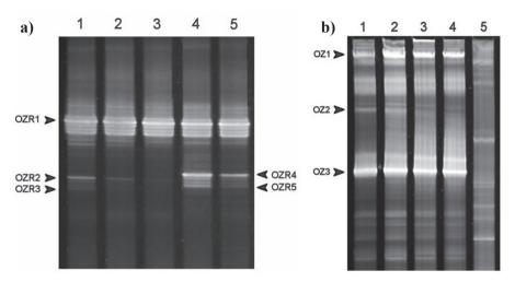
Fig. 2. DGGE gel with MBR activated sludge samples under anoxic conditions photographed in UV light for (a) 16S rRNA gene PCR products (b) *amoA* gene PCR product. Characteristics of species corresponding to labeled bands are given in Table 2
