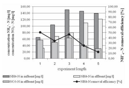
Fig. 1. Nitrogen compounds concentration and ammonia oxidation effectiveness measured for MBR bioreactor during the experiment; NO<sub>2</sub> concentrations in the effluent not shown due to a very low values obtained
