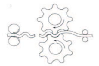
Fig. 1. Scheme of continuous RCS method [17]
