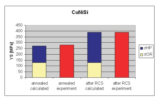
Fig. 9. Comparison of yield strength value calculated and obtained in experiment for CuNiSi alloy
