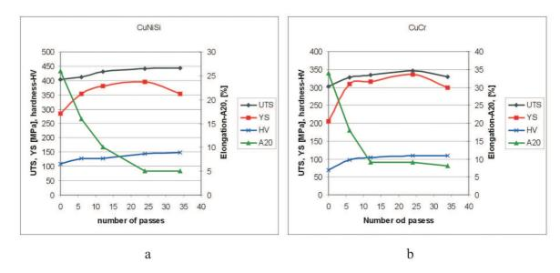
Fig. 7. Changes of mechanical properties of CuNiSi (a) and CuCr (b) strip during CRCS processing
