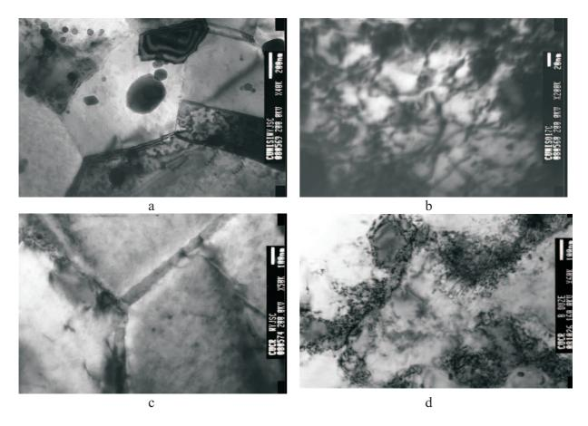
Fig. 6. Microstructure of CuNiSi alloy strips: as annealed (a), after 34 passes of deformation (b); and CuCr alloy strips: as annealed (c), after 34 passes of deformation (d); TEM
