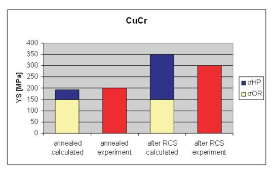
Fig. 8. Comparison of yield strength value calculated and obtained in experiment for CuCr alloy
