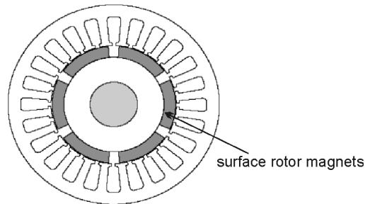
Fig. 1. SPMSM rotor assembly
