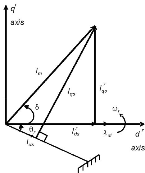
Fig. 6. Stator input current phasor diagram
