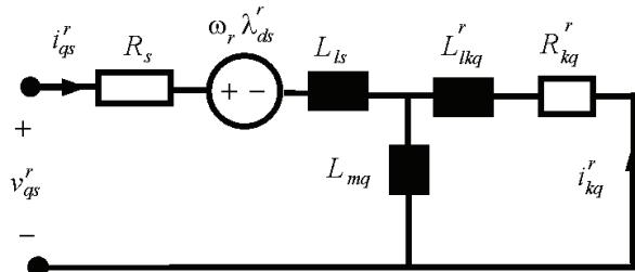
Fig. 3. *q*-axis equivalent circuit
