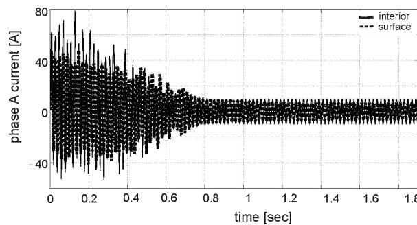
Fig. 11. Stator current transient at no load
