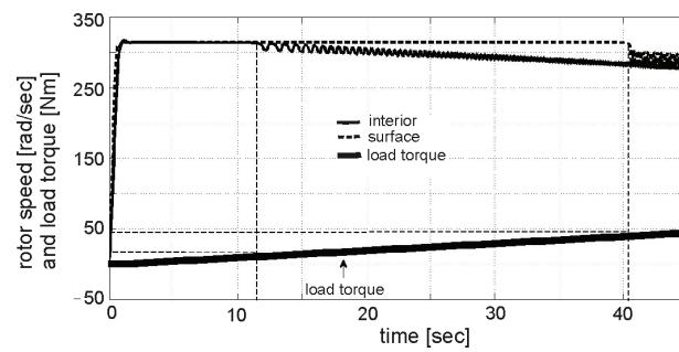
Fig. 13. Speed dynamics with ramp loading
