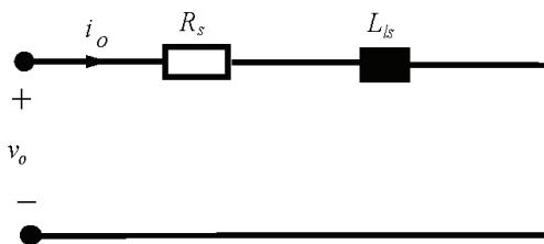
Fig. 5. Zero-sequence equivalent circuit
