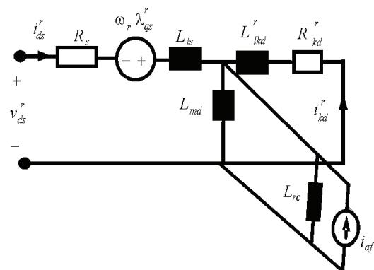
Fig. 4. *d*-axis equivalent circuit
