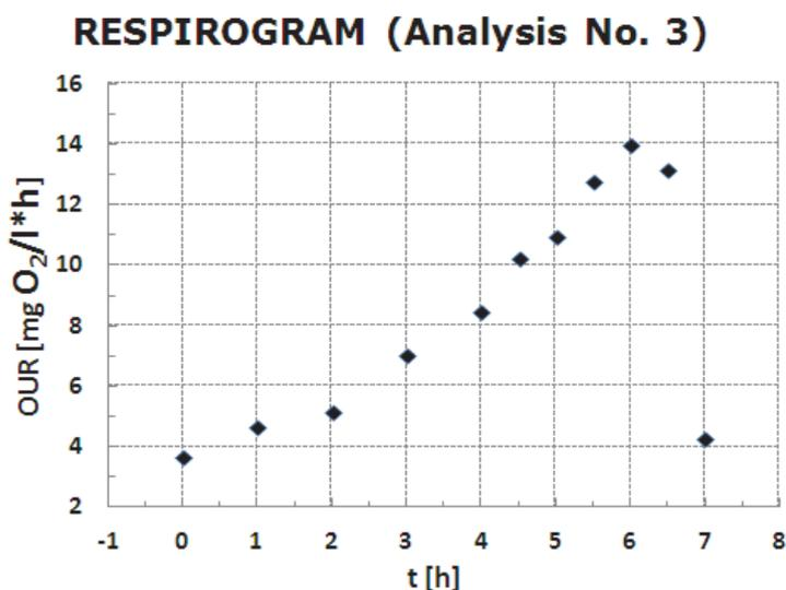
Fig. 3. Representative respirogram obtained during estimation of half saturation coefficient for organic substrate ( $K_S$ ) and maximum specific growth rate of heterotrophic biomass ( $\mu_{max}$ ). The decline in  $OUR$  value (at about seventh hour of the test) corresponds to expiration of a readily biodegradable soluble organic matter in the batch reactor (Trojanowicz et al., 2009)
