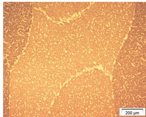
Fig. 1. Aluminium bronze, water cooled from the liquid state. Nucleation of  $\alpha$  phase (white) at the grain boundaries; at the grain centre  $\beta$ -phase (x 450)
