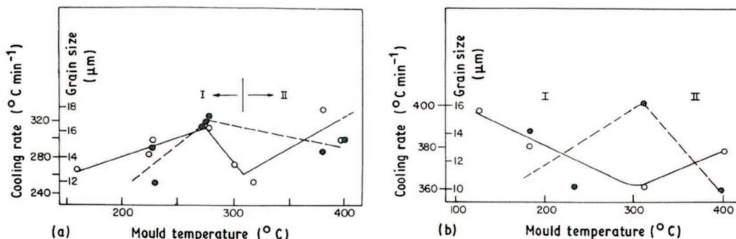
Fig. 8. The interdependence of the cooling rate (●) and  $\alpha$  grain size (○) as a function of the pre-heating temperature of the die. (a) Graphite coating thickness 0.01 mm; (b) Graphite coating thickness 0.1 mm
