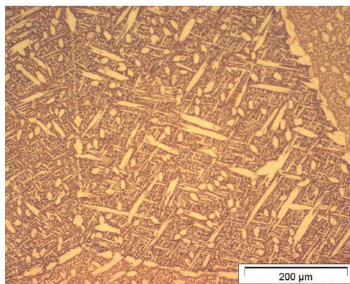
Fig. 5. Needle-shaped  $\alpha$  grains with emphasised boundaries, in casting made in a mould coated with graphite 0.10 thick (x 230)
