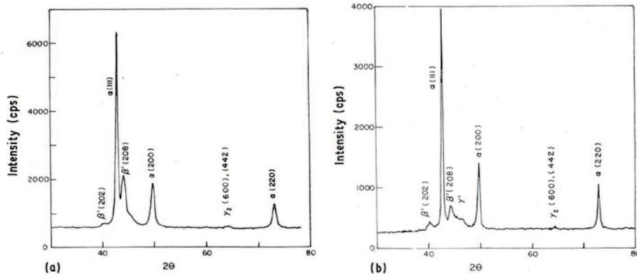
Fig. 6. X-ray diffraction of aluminium bronze. (a) No formation of  $\gamma'$  when casting into cold die. (b) Segregation of  $\gamma'$  when casting into hot die followed by slow rate solidification
