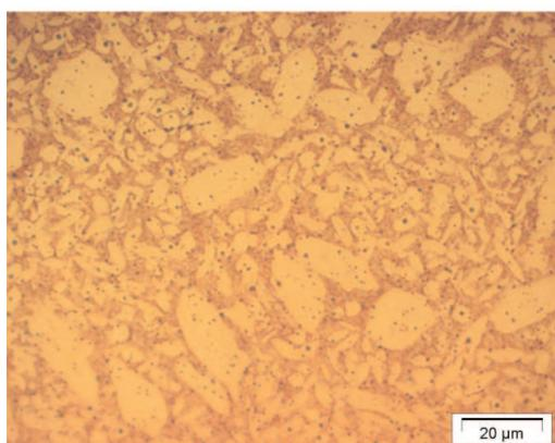
Fig. 4. Highest cooling rate, spherical  $\alpha$ , die pre-heated to 280°C. Graphite coating thickness 0.01 mm (x 360)
