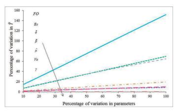
Fig. 7. Sensitivity analysis of the dimensionless temperature at  $\tilde{x}=0$  with respect to different parameters (Reference values:  $Ve=1, \gamma=0.1, Fo=0.1, g_0=100, \mu=5, \beta=1, \delta=5$ )
