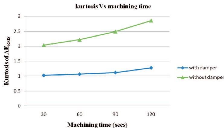
Fig. 8. Kurtosis of  $AE_{RMS}$  vs. machining time
