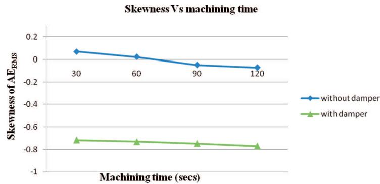
Fig. 9. Skewness of AERMS vs. machining time
