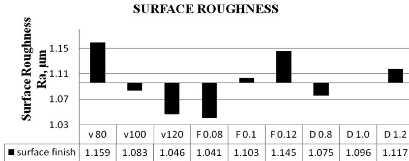
Fig. 6. Relative significance of input parameters on surface roughness
