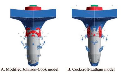
Fig. 8a. Failure patterns using different failure criteria (3 mm plate)
