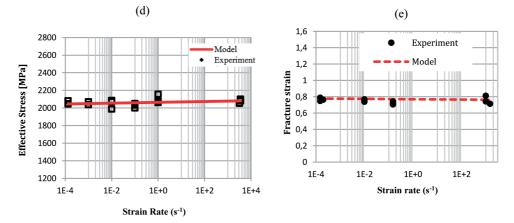
Fig. 3. Comparison between experimental data and model results for 30PM armour steel
