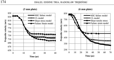
Fig. 11. Projectile velocity history during perforation of 30PM steel plates
