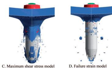
Fig.8b. Failure patterns using different failure criteria (3 mm plate) perforation tests on the 6 mm thickness plate showed that
