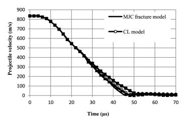
Fig. 12. Projectile velocity history during perforation of 8 mm thickness 30PM steel plates
