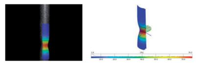
Fig. 2. True strain measurements during uniaxial tensile test using 3D deformation analysis
