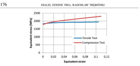
Fig. 14. Comparison between tensile and compression stress-strain curves of 30PM steel
