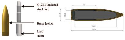
Fig. 4. Schematic drawing geometry of 7.62 mm AP bullet
