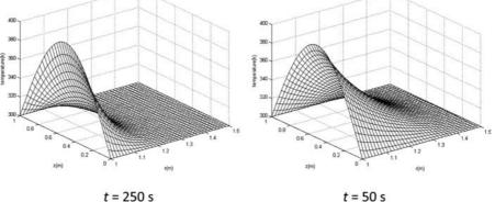
Fig. 3. Temperature distribution through the cylinder at different times for n = 5
