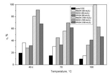
Fig. 2. The effect of temperature on single-stage extraction efficiency  $\eta$
