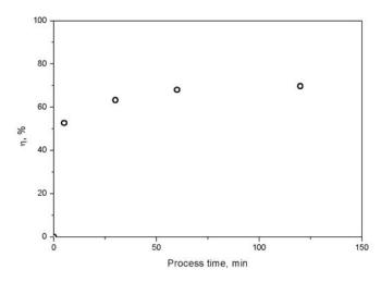
Fig. 7. Extraction efficiency  $\eta$  vs. process time (70 °C, 18 MPa)
