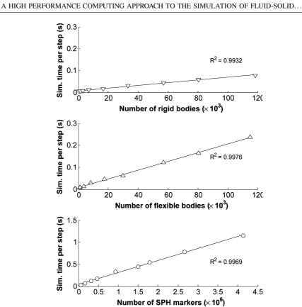
Fig. 5. Scaling analysis of Chrono::Fluid for rigid body dynamics, flexible body dynamics, and fluid dynamics as function of problem size  $(N_r, N_f, \text{ and } N_m, \text{ respectively})$ . The coefficients  $R^2$  are specified to each linear regression
