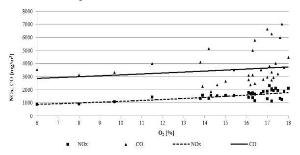
Fig. 2. Exhaust gases composition dependence from oxygen [%] during stabilized sludge combustion
