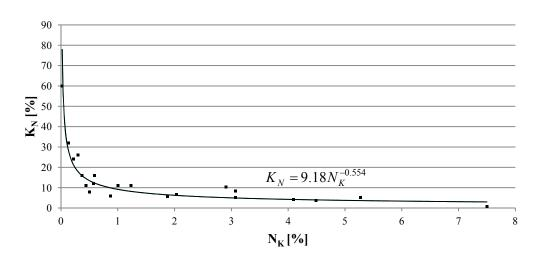
Fig. 10. Fuel nitrogen conversion factor to NO<sub>x</sub> dependence of the total nitrogen content in the fuel
