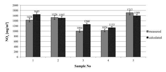
Fig. 12. Average concentrations of NOx, the investigation and the resulting calculations comparison; 1 – stabilized sludge; 2 – stabilized sludge with sawdust (ratio 50:50); 3 – stabilized sludge with sawdust (ratio 25:75); 4 – stabilized sludge with peat (ratio 50:50); 5 – untreated sludge
