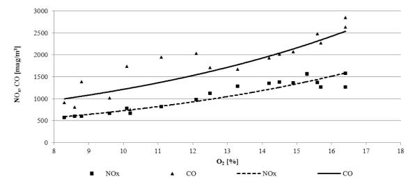
Fig. 5. Exhaust gases composition dependence from oxygen [%] during stabilized sludge and peat (ratio 50:50) combustion
