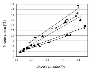
Fig. 11. NOx dependence from excess air ratio;
