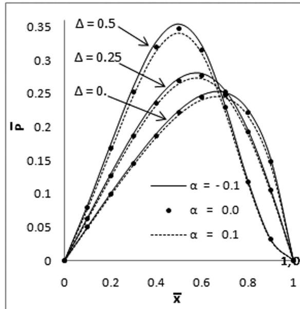
Fig. 2. Variation of dimensionless steady state film pressure ( $\bar{p}_0$ ) with dimensionless coordinate  $\bar{x}$  for  $r_b = 2$ . For  $\Delta = 0$  Newtonian results are identical with Taylor and Dowson [22] and other results are identical with Hsu and Saibel [6]
