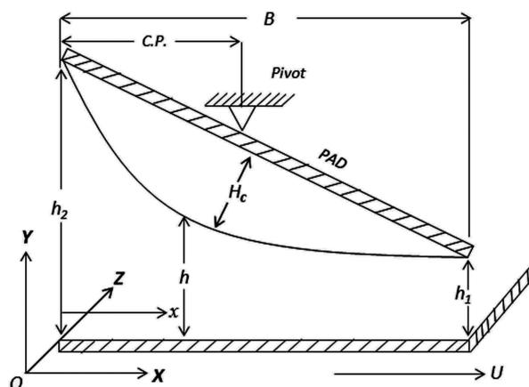
Fig. 1. Schematic diagram of curved slider bearing with a pivot at centre of pressure (C.P.).
