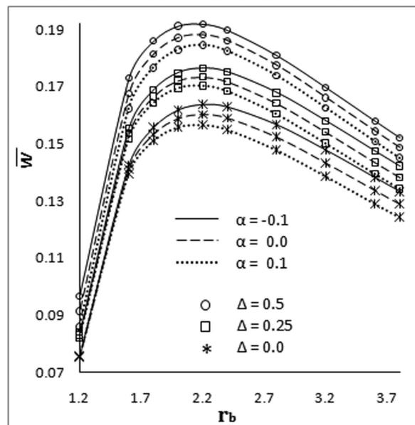
Fig. 4. Variation of dimensionless steady state load carrying capacity ( $\bar{W}$ ) of bearing with  $r_b$ . Newtonian results are identical with Kapur [20], and results for  $\Delta = 0$  are all identical with Hsu and Saibel [6]
