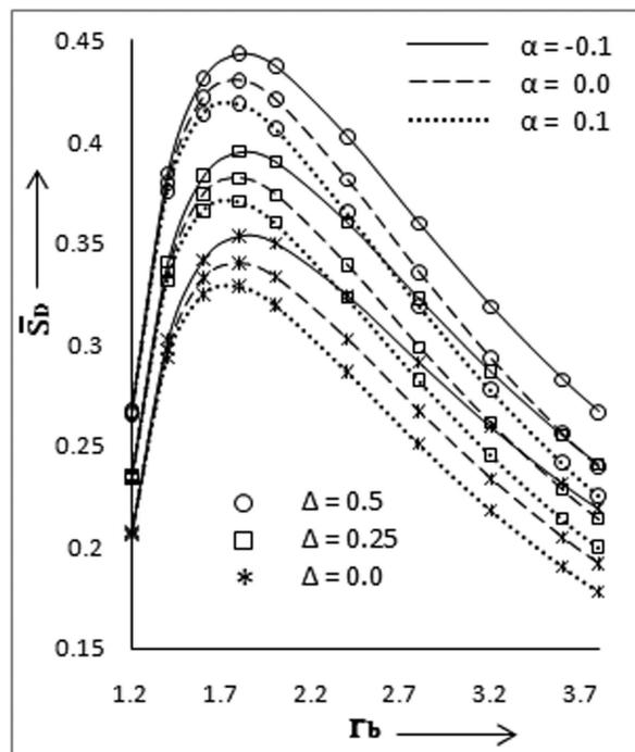
Fig. 6. Variation of dimensionless stiffness coefficient  $\bar{S}_D$  with thickness ratio  $r_b$  for different values of  $\alpha$
