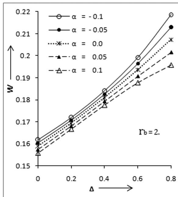
Fig. 3. Variation of dimensionless steady state load carrying capacity ( $\bar{W}$ ) of bearing with  $\Delta$  for  $r_b = 2$ . Newtonian results are identical with Kapur [20], and results for  $\Delta = 0$  are identical with Hsu and Saibel [6]
