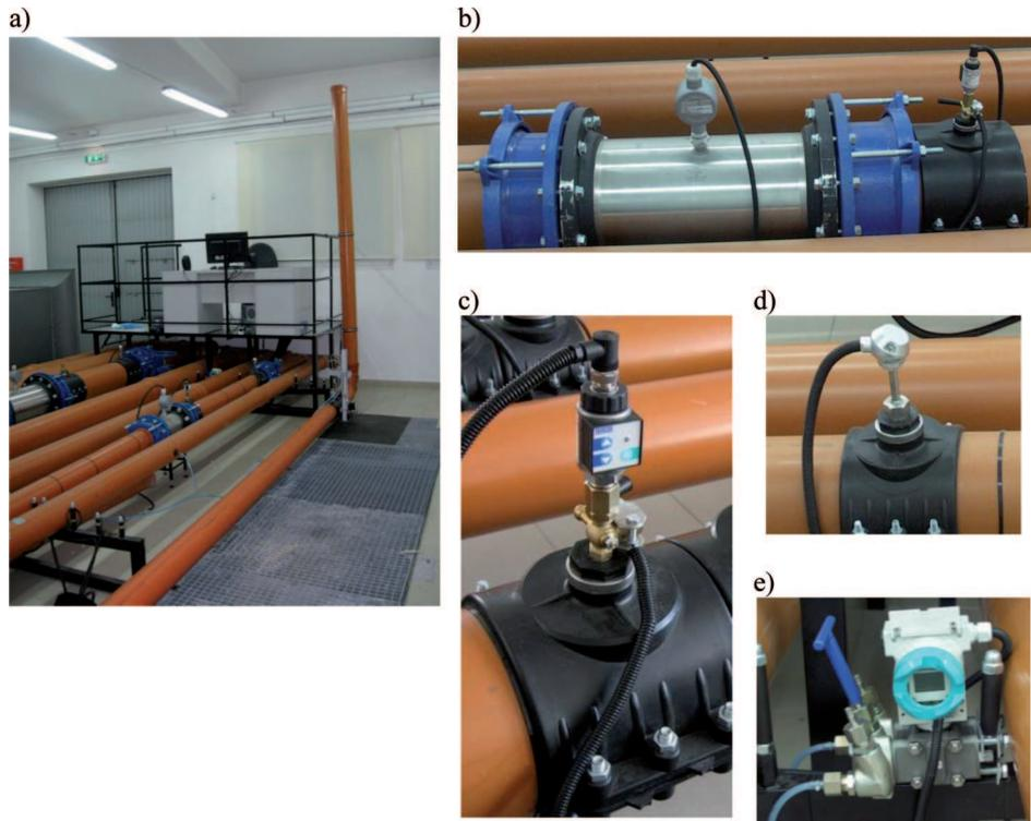
Fig. 3. Test stand for examining disturbances behind the segmented elbow: a) general view, b) turbine flowmeter, c) absolute pressure transducer, d) thermometer Pt-100, e) differential pressure transducer
