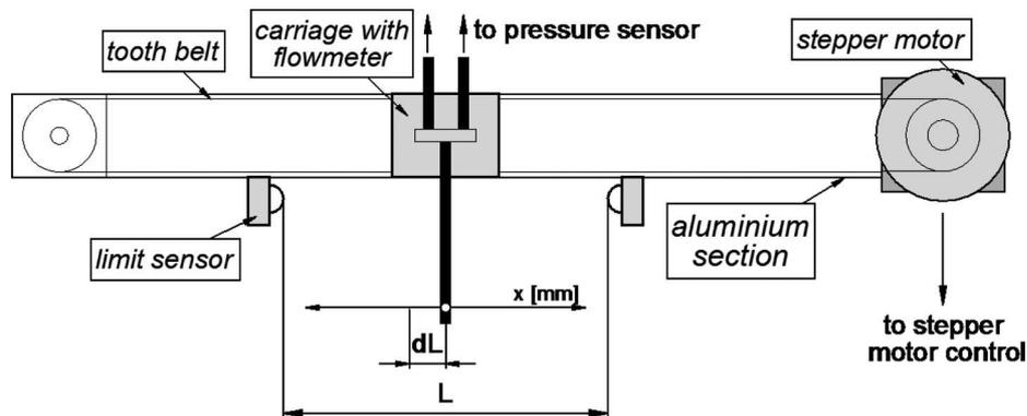
Fig. 5. Structure of the flowmeter movement system
