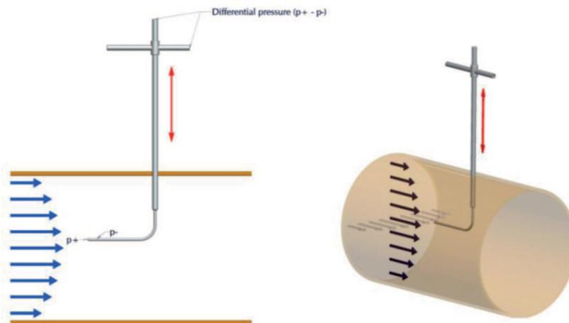
Fig. 1. The main idea for velocity profile measurement
