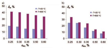
Fig. 9. Changes in the loop parameters at the temperature of 20 and 600°C: a)  $\delta_{\sigma}$ , b)  $\delta_{\varepsilon}$
