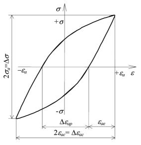
Fig. 2. Hysteresis loop and its basic parameters
