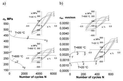
Fig. 6. Changes in the loop parameters at the level  $\varepsilon_{ac} = 0.35\%$ : a)  $\sigma_a = f(n)$ , b)  $\varepsilon_{ap} = f(n)$
