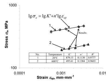
Fig. 10. Graph of strain for GX12CrMoVNbN9-1 cast steel
