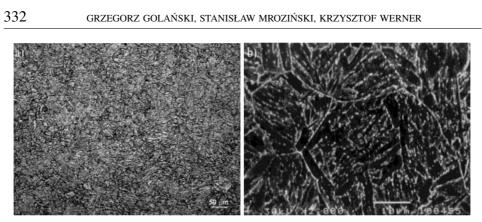
Fig. 3. Microstructure of GP91 cast steel in as - received state: a) OM; b) SEM; nital etched
