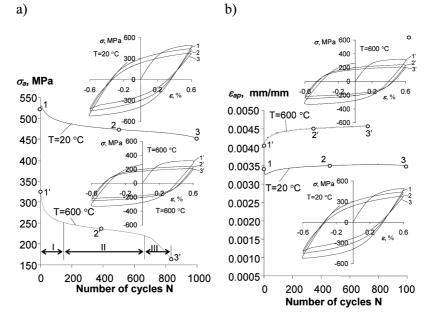
Fig. 7. Changes in the loop parameters at the level  $\varepsilon_{ac} = 0.60$  %: a)  $\sigma_a = f(n)$ , b)  $\varepsilon_{ap} = f(N)$
