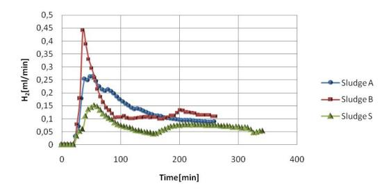
Fig. 4. The progress of hydrogen release during pyrolysis
