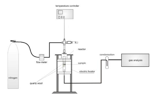
Fig. 2. Diagram of pyrolytic apparatus
