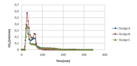
Fig. 3. The progress of carbon dioxide release during pyrolysis
