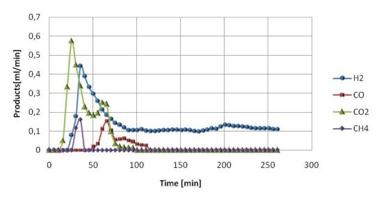
Fig. 5. The progress of gas releasing during pyrolysis of limed sludge B, CWWTP Ostrava
