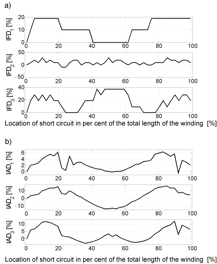
Fig. 8. Localization of one-turn short circuit along the winding: a) IFD_i and b) IAD_i
