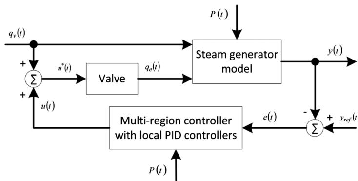
Fig. 1. Steam generator water level control structure.
