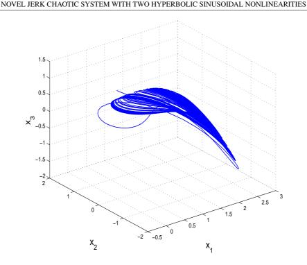
Figure 1. Strange attractor of the Sprott jerk system
