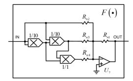
Figure 12. Designed electronic circuit modeling of the inverting hyperbolic sinusoidal block. Here the values of components are selected as:  $R_{n1} = 10k\Omega$ ,  $R_{n2} = 1M\Omega$ ,  $R_{n3} = 60k\Omega$ , and  $R_{n4} = 120k\Omega$
