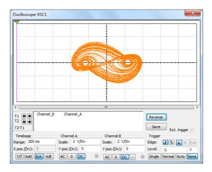
Figure 13. 2-D projection of the designed electronic circuit on  $(x_1, x_2)$ -plane obtained from NI Multisim.
