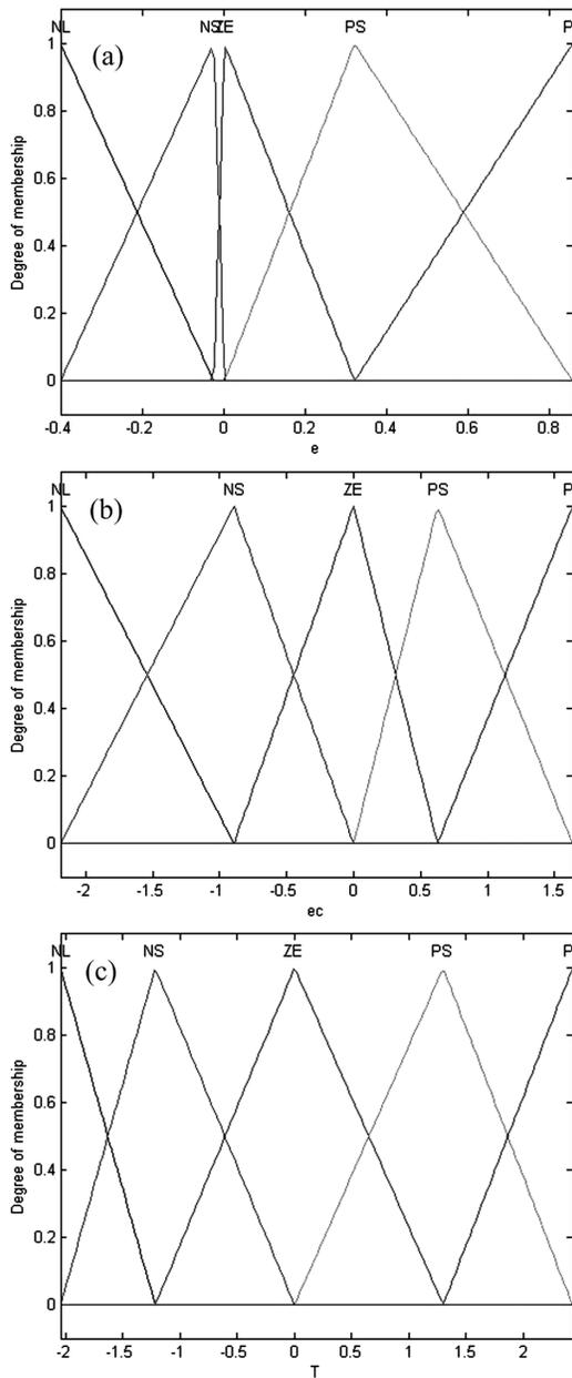
Figure 10. BFO optimized FLC membership functions: (a) E, (b) CE, (c) T.
