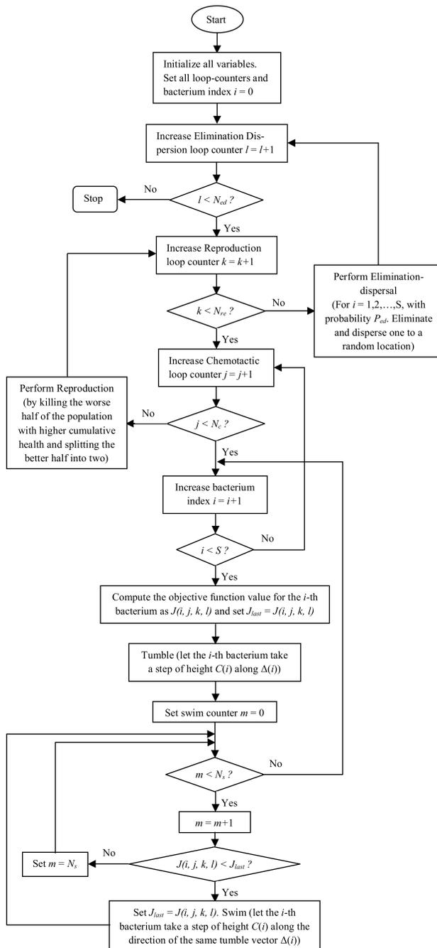
Figure 7. BFO algorithm.
