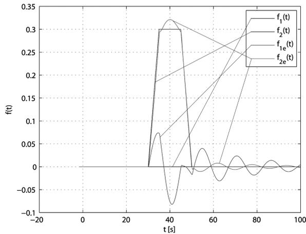
Figure 1. The second actuator fault and its estimation
