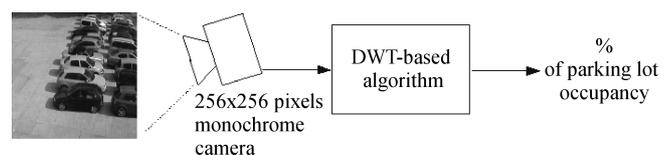
Fig. 1. The block diagram of the proposed system
