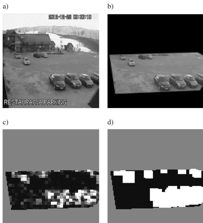
Fig. 2. Images illustrating selected steps of the algorithm, a) input image of the parking lot, b) region of interest of the input image, c) Combined 2D DWT scale images (result of the step 3), d) Previous image after applying the threshold and morphological operations (result of the step 4 and 5)
