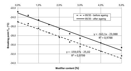
Fig. 2. Graphical presentation of Fraass breaking point for bitumen 95/35 and its varieties with addition of "modifier A" before and after ageing by RTFOT for the data presented in Table 2
