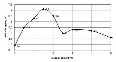
Fig. 4. Dependence between the increase of plasticity range ( $\Delta PR$ ) after ageing and "modifier A" content in bitumen 95/35 (for data from table 3)
