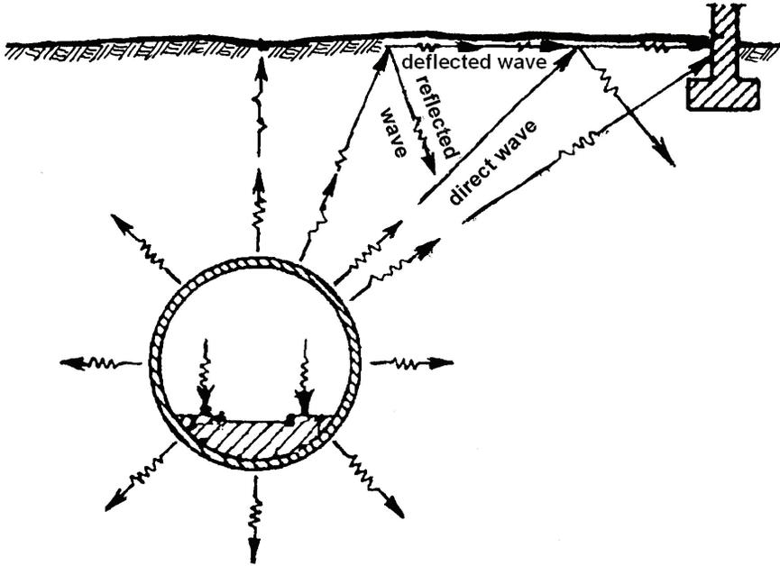
Fig. 4. Scheme of wave propagation from the underground tunnel to the surface of the ground
