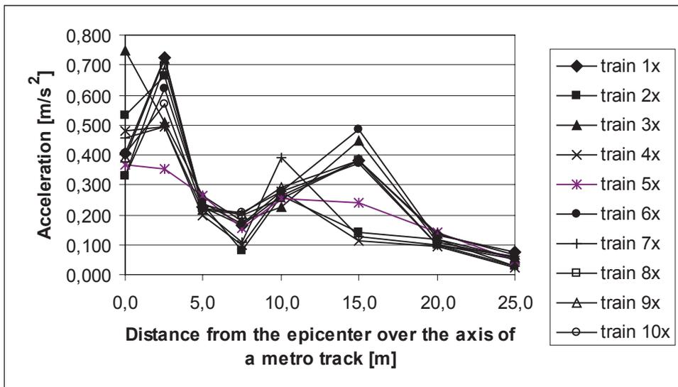
Fig. 7. Propagation of the ground surface vibrations caused by underground train passages in tunnel – distribution of acceleration amplitudes for horizontal radial component x (direction perpendicular to the underground tunnel)
