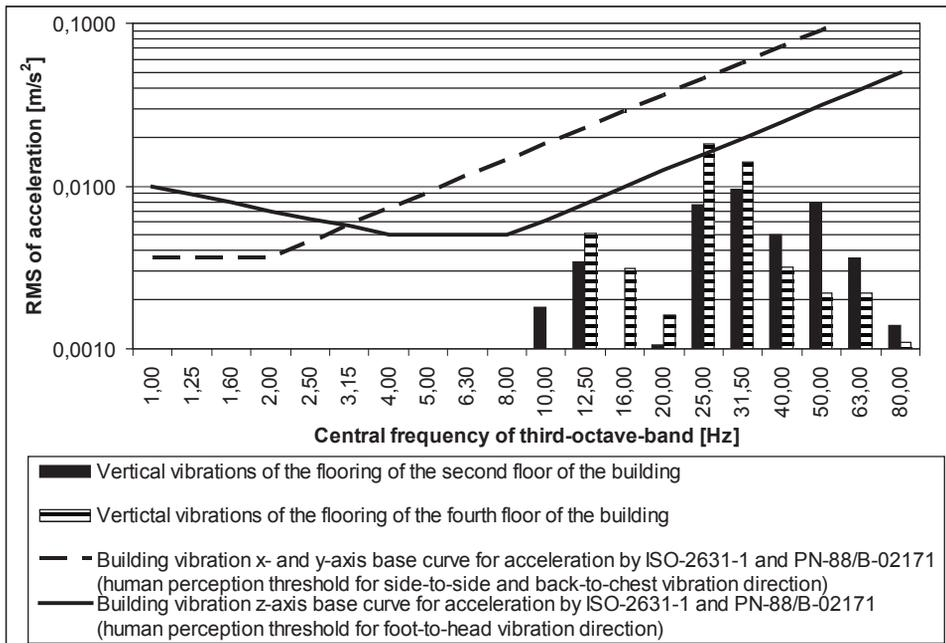
Fig. 17. Results of analyzes of the influence of vertical vibration on people living on the second and the fourth floor of the building I-10 in the case of vibrations caused by tramway passage 9 meters from the building
