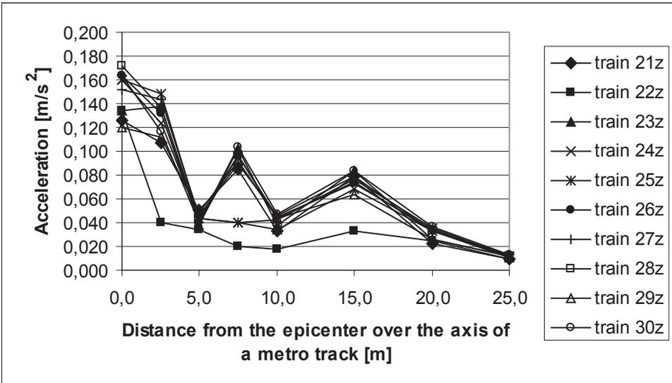
Fig. 9. Propagation of the ground surface vibrations caused by underground train passages in tunnel – distribution of acceleration amplitudes for vertical component z
