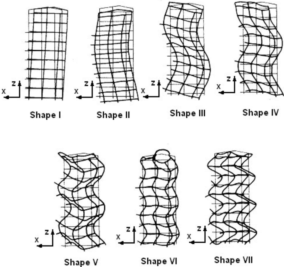
Fig. 14. Vibration shapes of a chosen frame of building B
