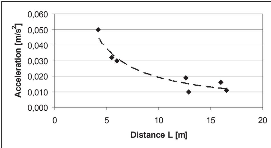
Fig. 12. Vibrations of the building in the ground level – dependence of acceleration amplitudes of vertical component  $z$  on the distance of the building foundations from the tunnel walls  $L$
