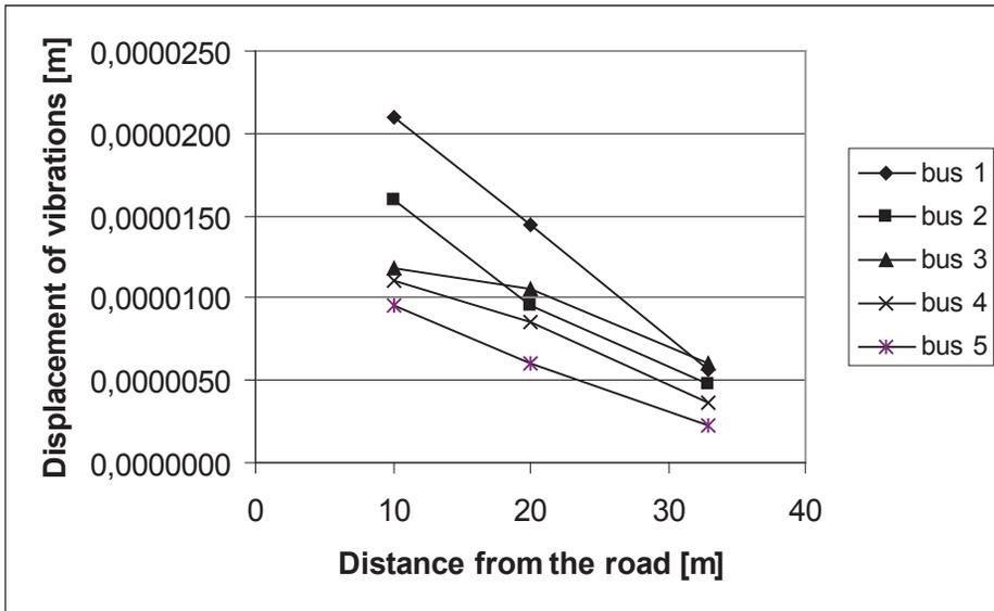
Fig. 2. Dependence of maximum amplitudes of the radial component  $x$  (horizontal component in the direction perpendicular to the road) of the ground vibration displacements caused by buses crossing from the distance from the road [5]
