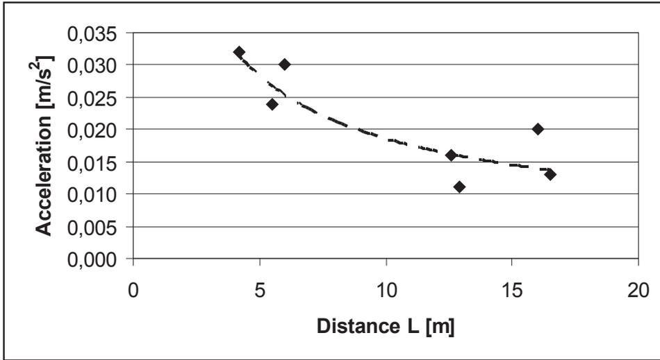
Fig. 11. Vibrations of the building in the ground level – dependence of acceleration amplitudes of horizontal radial component  $x$  (direction perpendicular to the underground tunnel) on the distance of the building foundations from the tunnel walls  $L$
