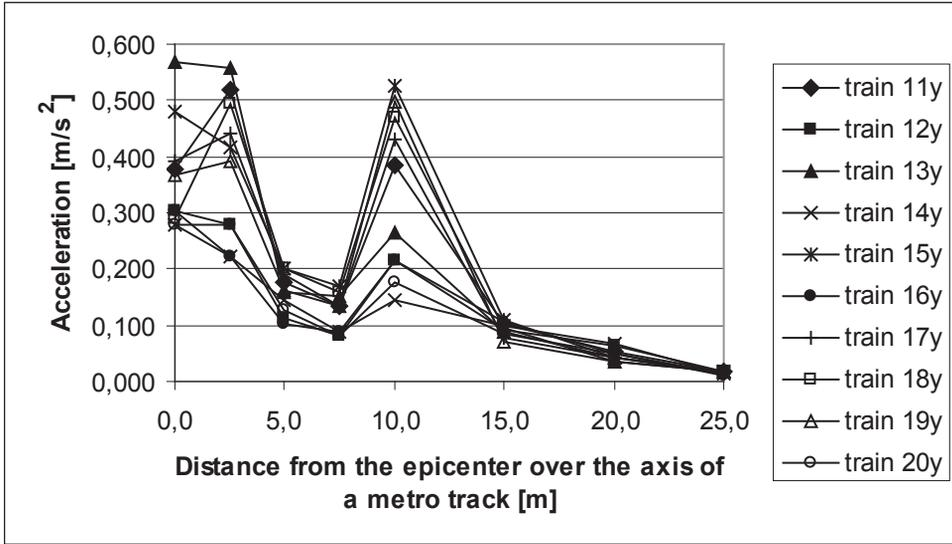
Fig. 8. Propagation of the ground surface vibrations caused by underground train passages in tunnel – distribution of acceleration amplitudes for horizontal transverse component y (direction parallel to the underground tunnel)
