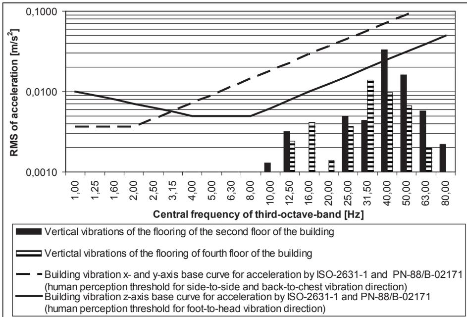
Fig. 16. Results of analyzes of the influence of vertical vibration on people living on the second and the fourth floor of the building I-10 in the case of vibrations caused by underground train passage in a tunnel 25 meters from the building
