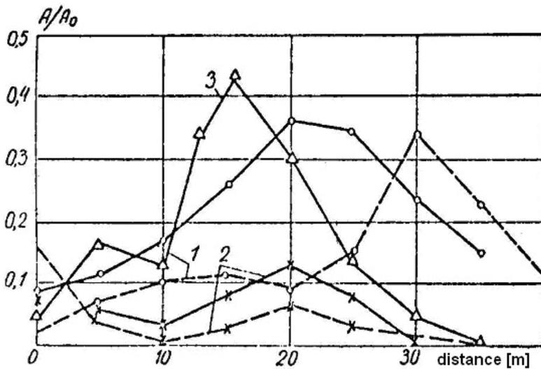
Fig. 5. Distribution of amplitudes of vertical and horizontal vibrations of ground surface by Czernobaj and Szatkowski [6]: 1 – precast reinforced concrete structure of the tunnel at forcing frequency  $f = 35$  Hz, 2 – as above at  $f = 70$  Hz, 3 – for monolithic reinforced concrete structure at  $f = 43$  Hz
