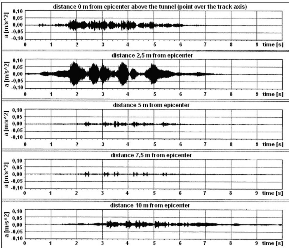
Fig. 6. Time-traces of the horizontal radial component  $x$  (in the direction perpendicular to the underground tunnel) of acceleration of the surface ground vibration caused by passage of the train (in underground tunnel) and registered in distances 0, 2.5, 5.0, 7.5 i 10 meters from epicenter over the axis of the underground track
