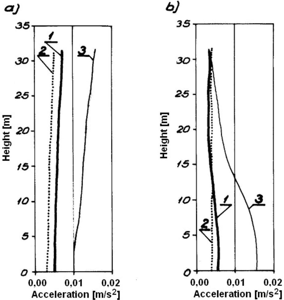
Fig. 15. Distribution of values of absolute acceleration with respect to building height for a) forcing by bus passage and b) forcing by underground train passage in the tunnel: 1 - horizontal radial component x, 2 - horizontal transverse component y, 3 - vertical component of floor vibration z
