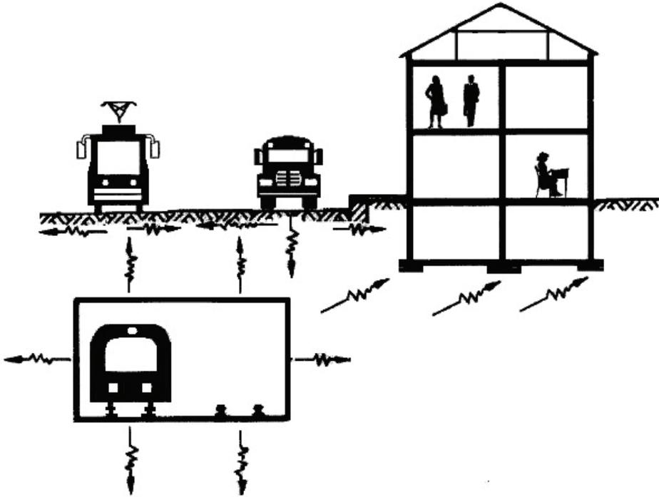
Fig. 1. Transmission of waves generated in a underground tunnel and caused by the surface transport to the building
