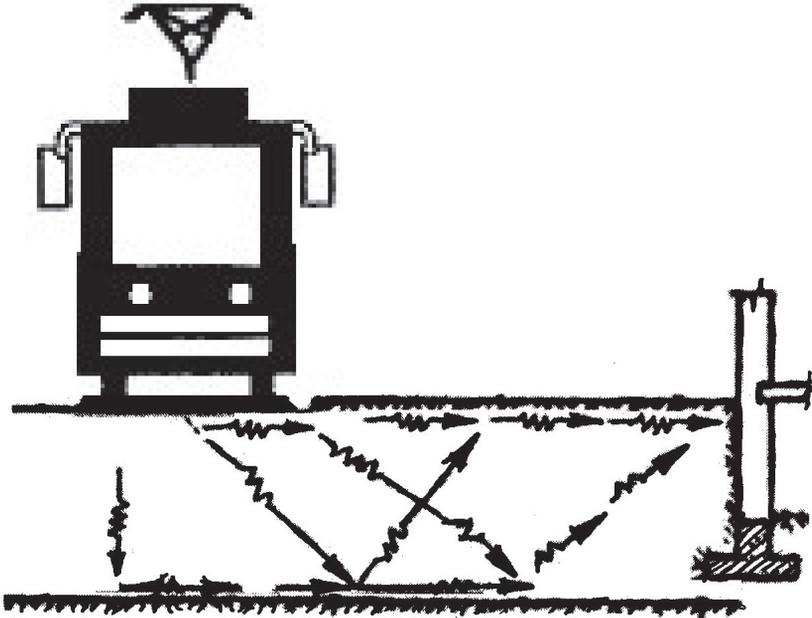
Fig. 3. Scheme of propagation in layered ground of waves caused by the surface source of the transport vibrations
