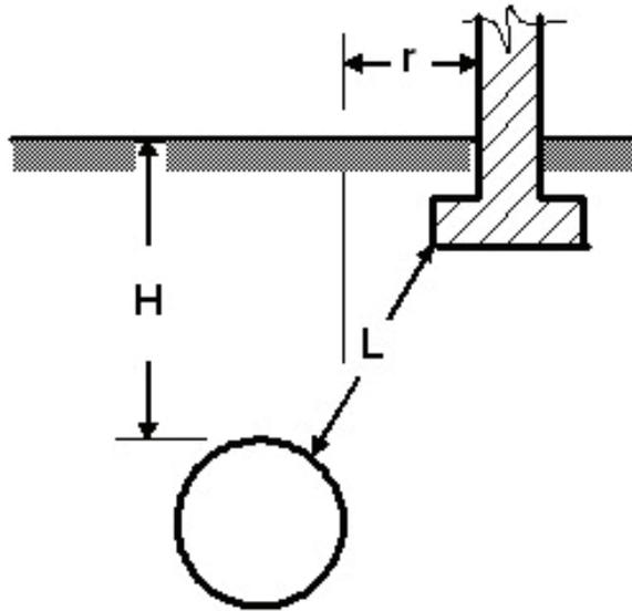
Fig. 10. Scheme of the position of the tunnel relative to the building
