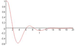
Fig. 5. The response of the system for  $b_1 = \tau = 7$ ,  $b_2 = 6$ ,  $c_2 = 0$ ,  $c_1 = 1$  and calculated  $c_3$  and  $c_4$  (the region of two real roots and one pair of complex-conjugate roots)
