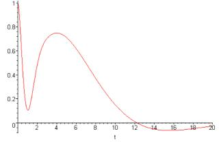
Fig. 7. The response of the system for  $b_1 = \tau = 4$ ,  $b_2 = 10$ ,  $c_2 = 0$ ,  $c_1 = 1$  and calculated  $c_3$  and  $c_4$  (the region of two pairs of complex-conjugate roots)
