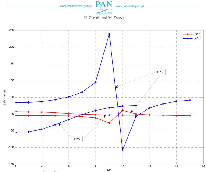
Fig. 4. Calculated values of  $\frac{c_3}{c_1}$  and  $\frac{c_4}{c_1}$  as a function of  $b_2$  for desired  $b_1 = \tau$  (the region of two real roots and one pair of complex-conjugate roots)
