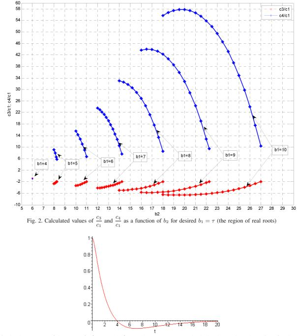
Fig. 3. The response of the system for  $b_1 = \tau = 7$ ,  $b_2 = 14$ ,  $c_2 = 0$ ,  $c_1 = 1$  and calculated  $c_3$  and  $c_4$  (the region of real roots)
