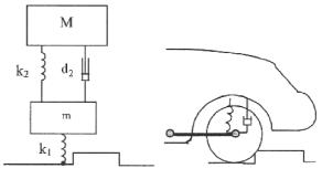
Fig. 8. Model of the suspension system
