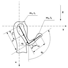
Fig. 1. Two-link arm in vertical plane
