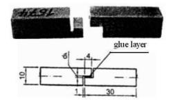
Fig. 3. Shape of a specimen in shear tests after [31] (Kubieniec [3]).
