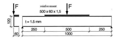
Fig. 14. Test arrangement for a reinforced beam from U profile, PASTERNAK, SCHWARZLOS, SCHIMMACH [10].
