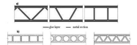
Fig. 19. Different cross-sections of hollow plates with thin (a) and thick (b) layers Feldman, Volling,  $Ge\beta$ ler, Wellershoff,  $Gel\beta$ , Wagner [8].
