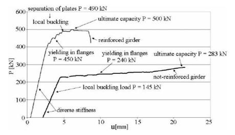
Fig. 18. Comparison of experimental P – u paths of equilibrium of the reinforced and not reinforced box girders PASTERNAK, KUBIENIEC, PIEKARCZYK [5], [21].
