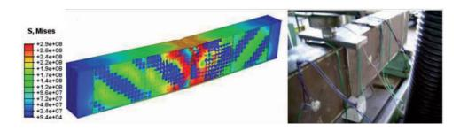
Fig. 10. Numerical (ABAQUS) and experimental models of a reinforced box – girder in the phase of failure PASTERNAK, KUBIENIEC, PIEKARCZYK [5], [21].
