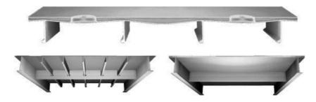
Fig. 20. Examples for the use of SPS – structures from shipbuilding (above) and bridge construction (bottom right, bottom left – conventional solution), FELDMAN, VOLLING, GE $\beta$ LER, WELLERSHOFF, GEI $\beta$ , WAGNER [8].
