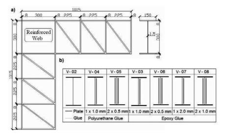
Fig. 15. Geometry and layouts of reinforcements of the knee joint, [5], [21].
