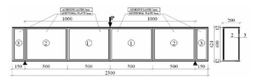
Fig. 17. Geometry and layouts of reinforcements of the box girder PASTERNAK, KUBIENIEC, PIEKARCZYK [5], [21].
