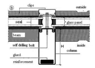
Fig. 12. Example of a beam-column supporting system of a façade - structural details, MEINZ [2].
