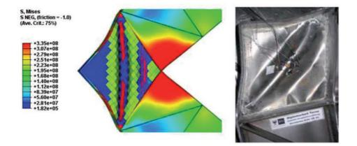
Fig. 9. Numerical (ABAQUS) and experimental models of a reinforced knee joint of a frame in the phase of failure PASTERNAK, KUBIENIEC, PIEKARCZYK [5], [21].
