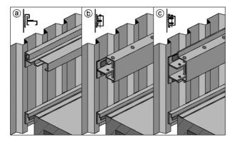
Fig. 11. Alternative ways of bonding of the folded sheet façades to the skeleton with use of adhesives, MEINZ [2].
