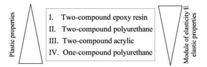
Fig. 1. Elastic and plastic properties of adhesives according to Table 1.
