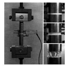
Fig. 5. Tensile test for an adhesive specimen after [33] (MEINZ [2]).
