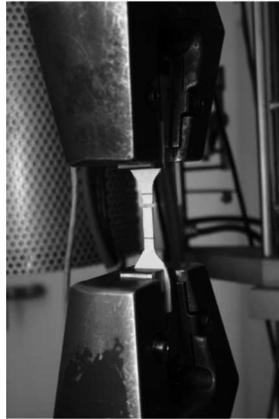
Fig. 4. Tensile test. failure of a specimen after [32] (KUBIENIEC [3]).
