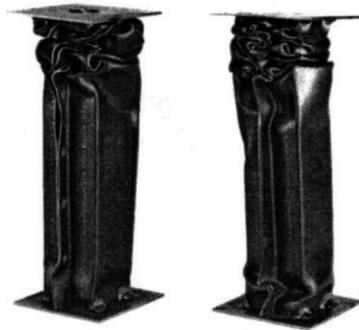
Fig. 13. Crash-tested double hat- profile, PASTERNAK, SCHWARZLOS, SCHIMMACH [10].
