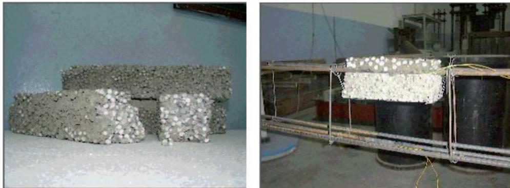
Fig. 2a. Mortar blocks representing honeycombs
